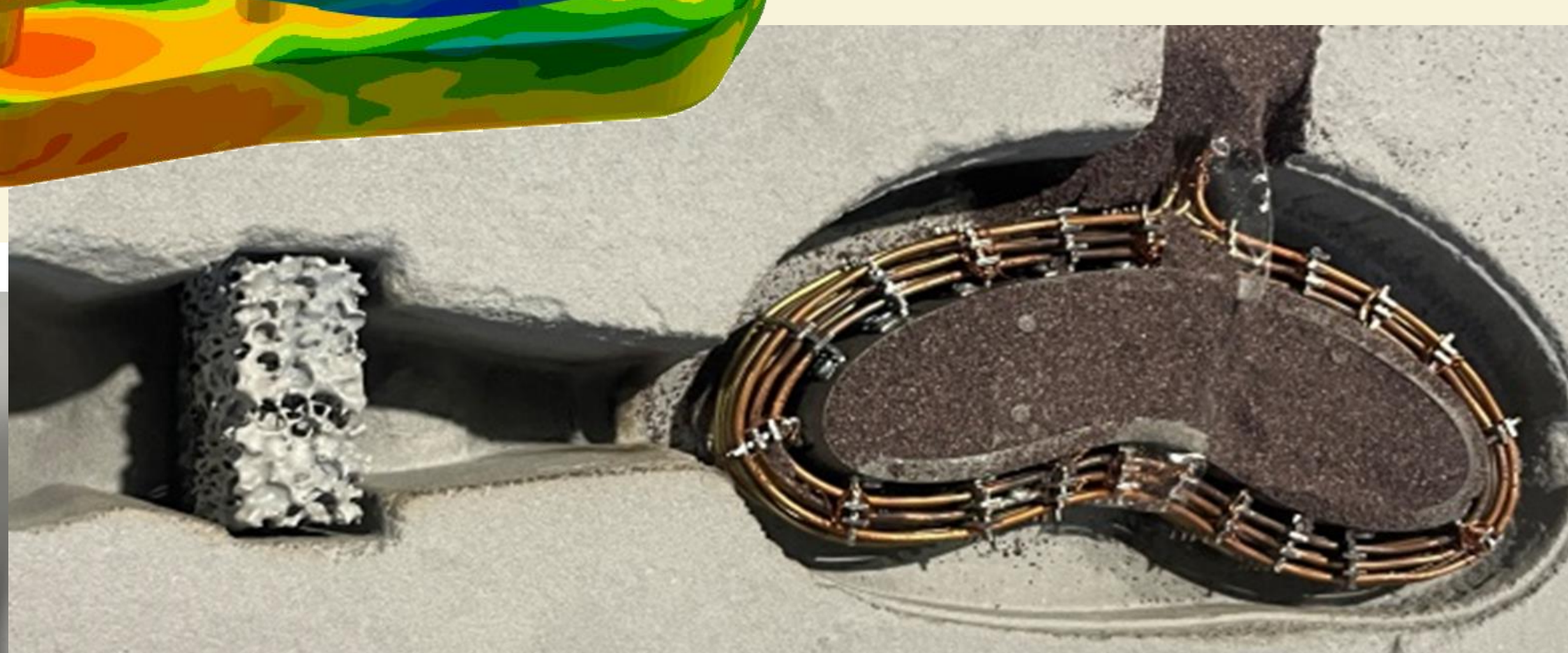
Sand mould compacted with organic binder, form, conductors, casting filter and sand inside the form core; prepared for casting in URKOASE S.L.
